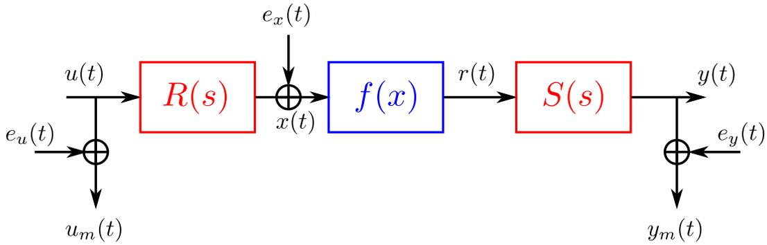
Figure 1: A Wiener-Hammerstein system with process noise. The LTI blocks at the input and the output are depicted by  $R(s)$  and  $S(s)$  respectively.  $f(x)$  denotes the static nonlinearity. The process noise  $e_x(t)$  enters the system before the static nonlinearity. Two smaller (neglectable) noise sources  $e_u(t)$  and  $e_y(t)$  are present in the measurement channels.  $u_m(t)$  and  $y_m(t)$  are the measured input and output signals.
